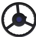
Steering wheel actuator 171mm x 65mm Rated voltage 12 VDC Rated current 3A Rated torque power 7-16 N.m Peak current 15A
